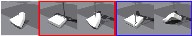
Fig. 2: Importance of manipulation point (MP) selection. Leftmost: goal shape; Red box: successful MP; Blue box: failed MP.
