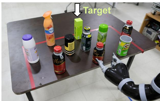
**Fig. 1** A dense clutter of 10 objects (the light green cuboid in the back is the target) in the 36 cm × 72 cm space marked by the red lines on the table. A subset of obstacles needs to be rearranged to retrieve the target. This is one of the instances that our method can provide a solution for
